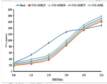
Fig. 8 Effect of BMEP on NOx
